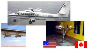
Figure 2: Twin-Otter and Droplet Particle Measuring Probes (on aircraft and in tunnel)
